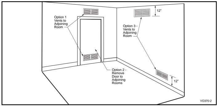
Fig. 4 Vent options to provide additional air.
